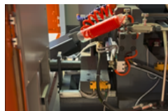
Third Vise Feature to minimise end-piece length
